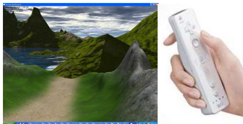
Fig. 1. A typical Direct-X landscape scene which the Wii remote-equipped patient can fly-through via slight wrist movements adjusted to the patient's abilities. Orientation sensitive accelerometers allow all of the processing to be done in the Wii remote and sent to the console via a blue tooth wireless channel; no line-of-sight required.
